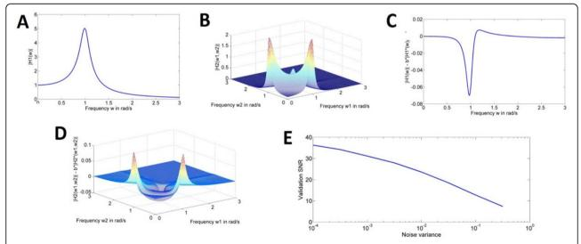
Figure 1 A&B - GFRF functions of the original filter, C&D - Difference between the original GFRFs and the scaled versions for the identified filter, E - SNR between the validation signal and the identified filter output.
