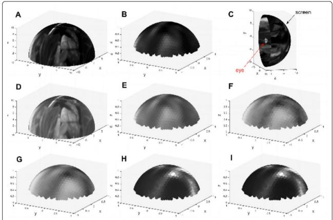
**Figure 1 A. Stimulus presented on a hemisphere screen**. B. Inputs (Number of Photons) to R1 photoreceptors in all ommatidia. C. Geometric relation between eye and screen. D. Gamma corrected screen intensity. E. Gamma corrected inputs to R1 photoreceptors. F. Voltage response of R1 photoreceptors. G. Averaged voltage response of photoreceptor terminals in all cartridges. H. Response of L1 neurons in all cartridges. I. Response of L2 neurons in all cartridges.
