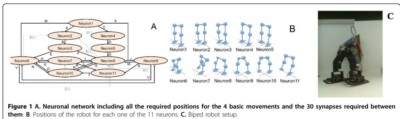
**Figure 1** A. Neuronal network including all the required positions for the 4 basic movements and the 30 synapses required between them. B. Positions of the robot for each one of the 11 neurons. C. Biped robot setup.
