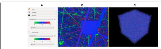
**Figure 1 Visualization Example.** The user interface widget shown in **(A)** dictates an example of the model-defined attributes being rendered for the connections (synapses) and neurons in addition to the current coloration for each attribute. An example of a 50,000 neuron, 250,000 synapse model is shown, close up **(B)** and from a distance **(C)**.
