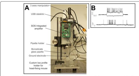
**Figure 1 (A) Single-channel patch chip amplifier in the patch clamping setup**. **(B)** Representative *in vivo* whole-cell recordings in current clamp mode using conventional pCLAMP software and the patch chip.
