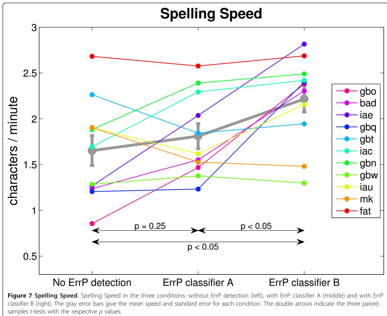
Tukey-Kramer post-hoc tests showed that spelling speed for classifier B was significantly higher than spelling speed without ErrP detection. The spelling speed obtained with classifier A did not differ significantly from the speed in the other conditions.
