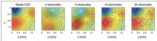
Figure 1 CSD reconstructions from randomly placed electrodes. Model data and reconstructions from 4, 8, 16, and 32 randomly placed electrodes
