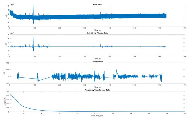
Fig. 2 Overview of the data of one planarian recorded during darkness along different processing stages. Raw data was imported into Matlab. In the next step, the raw data were filtered between 0.1 and 23 Hz to remove line noise artifacts. Subsequently, the data were cut into 6 s-segments, and noisy segments were removed. Finally, data were transformed into the frequency domain between 0.5 and 20 Hz
