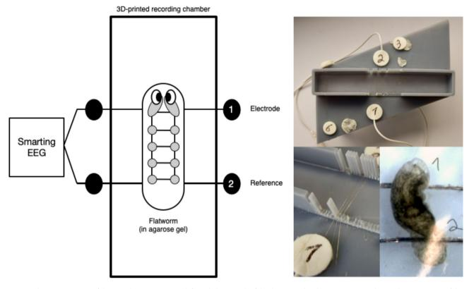
**Fig. 1** Schematic overview of the recording environment (left) and photograph of the device used in the experiments with one planarian on top of the electrodes (right). The animal is fixated in 2% agarose gel and placed on top of wire electroretinography electrodes. The electrodes are held in place in a 3D-printed recording chamber and are connected to a mobile EEG recording device
