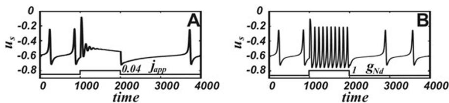
**Figure 1** The NMDAR activation elevates the frequency, while the applied depolarization blocks oscillations. The voltage time-series are shown in response to square pulses of the applied depolarization (A) and NMDAR activation (B).
